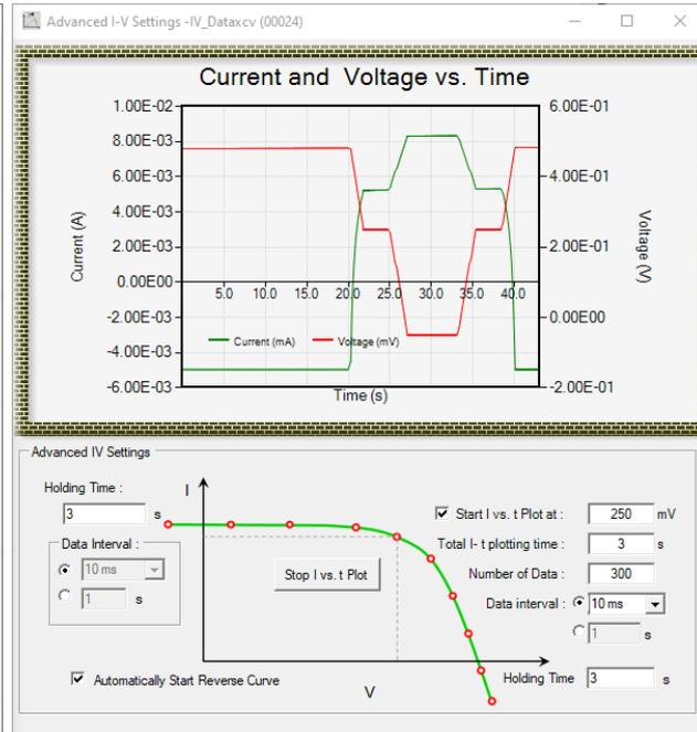
“Advanced IV Setup” allows user to change various settings such as “start” point holding time, “end” point holding time, current vs. time plot for each data point, and/or at given fixed voltage in the middle of I-V curve tracing.
