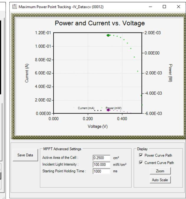
“Advanced MPP tracking” function shows the power, current, voltage and efficiency curves from the starting point of the MPP tracking so that user can see how it reach to maximum power point from different starting points and directions. It is continuously plot the conversion efficiency vs. time curve.
