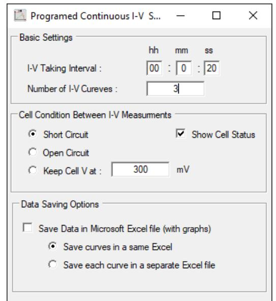
“Programmed Continuous IV” function allow user to take series of IV curves on given time intervals. User can also determine the cell keeping condition during I-V measurements. Data can be save in a single Excel file or separate files.
