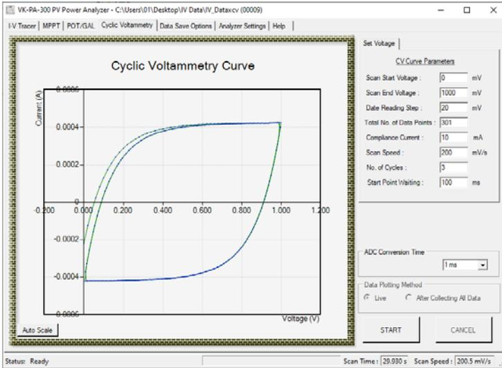
“Cyclic Voltammetry” allows user to get both three electrode and two electrode CV plots for given voltage range, scan speed and number of cycles.
