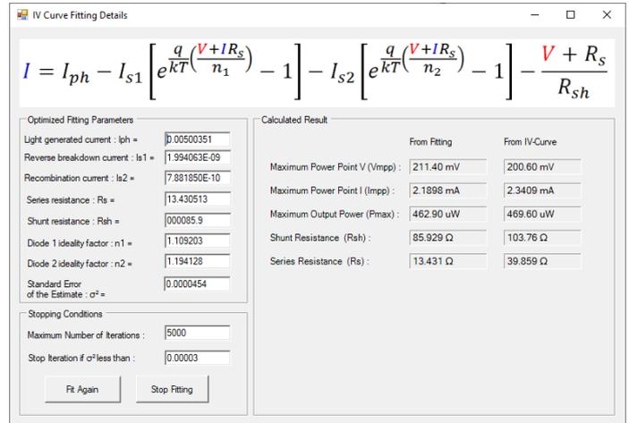
I-V curve fitting function automatically fit the I-V data with two diode model and calculate various parameter.
