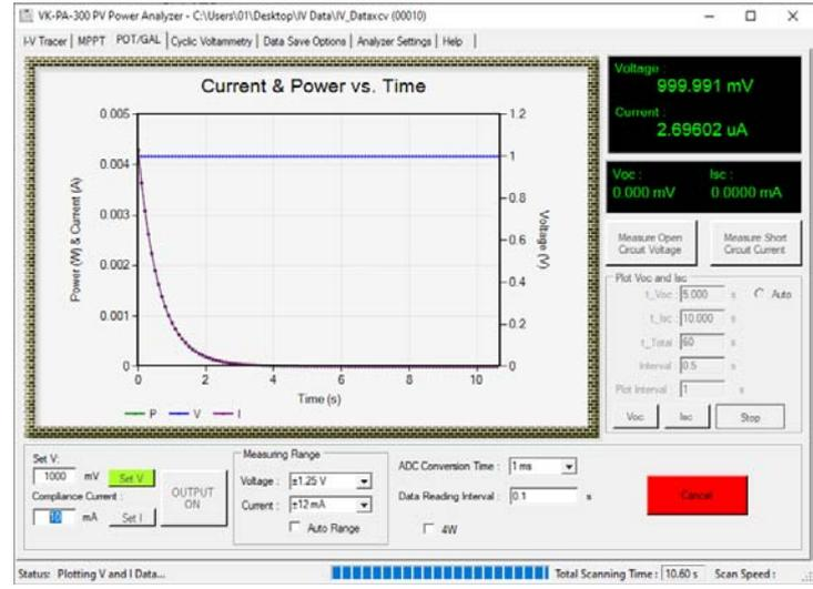
“POT/GAL” Tab allows user to set constant voltage or current to the sample and measure and plot data. Also Voc and Isc of solar cells can be measured with single click.
